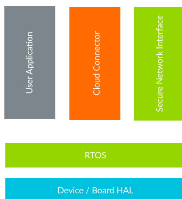
Fig. 1: IoT application components - simplified
